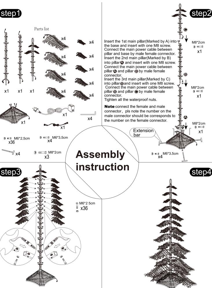
Insert the leaves into the leaf base from top to down. Note that the number on the leaf should corresponds to the number on the base. Number marked from #36 to #1.Pls note #36 should be corresponded to #36 hole,35-35 ...1-1. Then fixed by a M6 screw at the overlap and connect the power cord to the leaves by male female connector. Tighten all the waterproof nuts.
